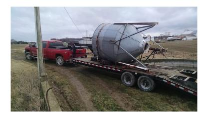
The bin in the picture below is the smallest of the three. We were able to transport it intact as it was 8 ft wide and 16 ft long. This holds 6 tons of grains and has a 100 ft flex auger to pump the grain out into feeding troughs. In this case, this bin was installed a confined feeding operation, so the flex auger was of use. For us, it will be spare parts in the barn.
